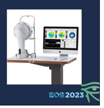
• Corneal densitometry (CD) software is implemented in the Scheimpflug corneal tomography system, providing numerical values on corneal densitometry and transparency.
